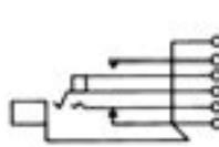
Tip closed; ring open circuits. Isolated switching—One "make" circuit.
