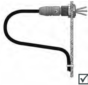
Empfohlene feste Installation Recommended fixed installation
